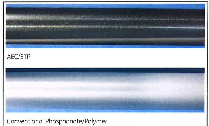
Calcium carbonate deposition studies under heat transfer conditions at 135°F (57°C), pH 8.6, 600 ppm Ca Hardness and LSI 2.5 for 6 Days.
